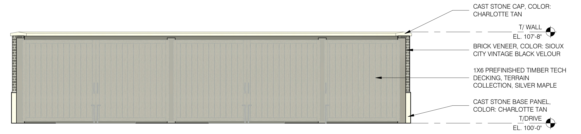
5 FRONT DUMPSTER ELEVATION SCALE: 1/4" = 1'-0"
