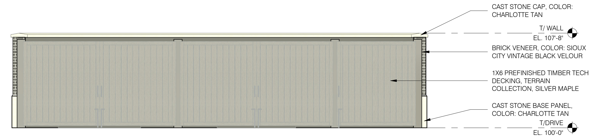
5 FRONT DUMPSTER ELEVATION SCALE: 1/4" = 1'-0"
